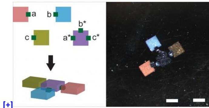
*Gel bricks smaller than a grain of salt (top left) can be programmed to self-assemble into complex structures. The key is to attach a pair of connector cubes coated with matching DNA glue on the gel bricks that are meant to pair up. (Credit: Wyss Institute)*
