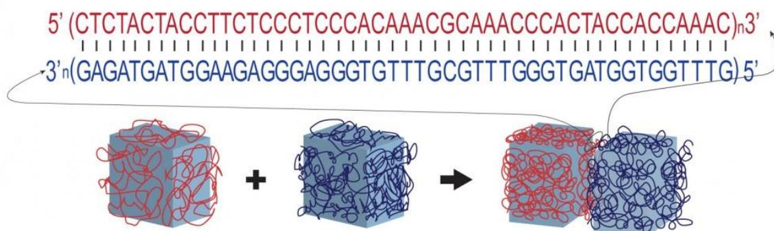
*DNA makes glue programmable because one strand of DNA will stick tightly to a matching partner strand, but only if the two strands have chemical "letters," or nucleotides, that are complementary (A to T, C to G). Gel bricks coated with matching strands of DNA adhere specifically to each other. (Credit: Wyss Institute)*
