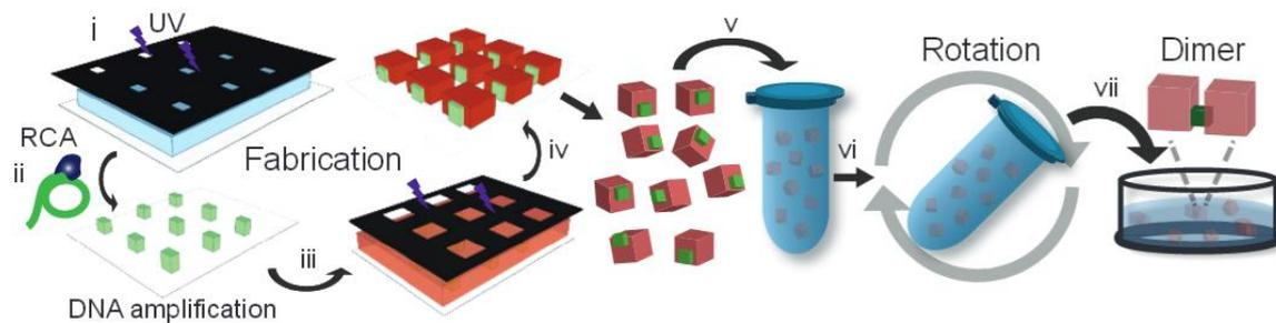
*Self-assembly of hydrogel cubes with face-specific DNA glue modifications: Hydrogel cubes carrying giant DNA glue on designated faces were fabricated in steps 1 – 4, collected in a 0.5 ml microtube in step 5, mixed and agitated in step 6, and transferred to a petri dish for imaging in step 7. (Credit: Wyss Institute)*
