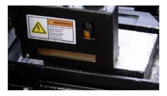
The printer works by having an inkjet spray a plastic binder over a bed of powder in layers of 20 microns, about half the width of a human hair. Following a computer's directions, it creates a channeled cylinder the size of a pencil eraser.
