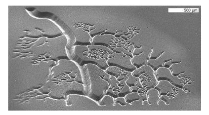
Printing three-dimensional blood vessels in seconds out of soft, biocompatible hydrogels (credit: Biomedical Nanotechnology Laboratory, Chen Research Group, UC San Diego Jacobs School of Engineering)
