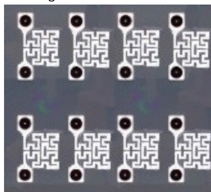
A Hilbert resistor array in a flip-chip package. Patent WO0154221
