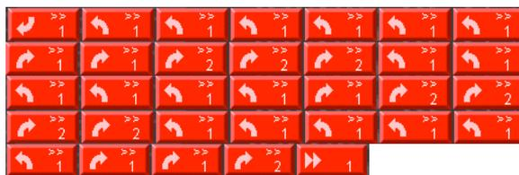
**Fig. 13.** The 32-step controller corresponding to the protein concentrations in Fig. 12 (read left to right). Note that the sequence partially repeats (up to command 18) before the robot reaches its destination.
