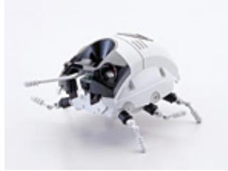
**Fig. 8.** The *wonderborg*<sup>TM</sup> robot (Bandai) has six legs, two feelers, two infrared collision detection sensors, a floor sensor, a light sensor and capabilities for the addition of a further motor and sensor.
