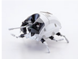
Fig. 8. The wonderborg TM robot (Bandai) has six legs, two feelers, two infrared collision detection sensors, a floor sensor, a light sensor and capabilities for the addition of a further motor and sensor.
