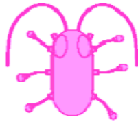
Fig. 8. The wonderborg TM robot (Bandai) has six legs, two feelers, two infrared collision detection sensors, a floor sensor, a light sensor and capabilities for the addition of a further motor and sensor.
